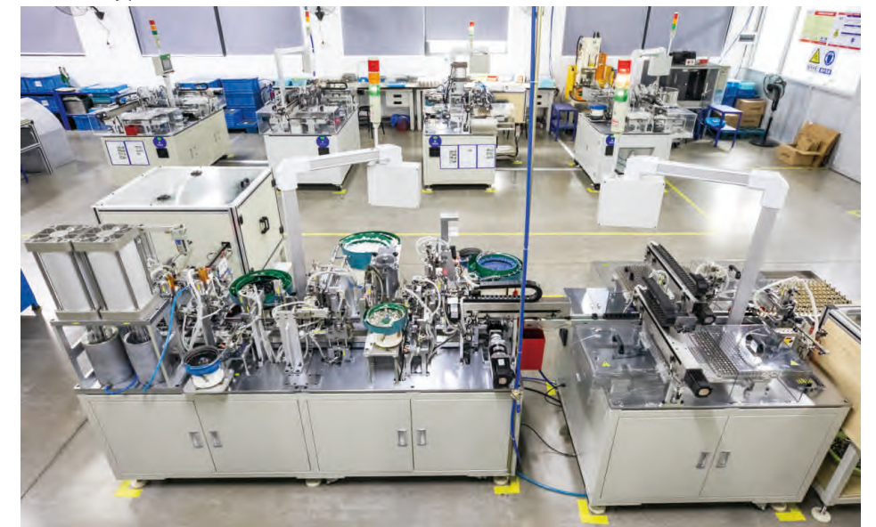
■ Automatic assembly line of pilot head for solenoid valves
