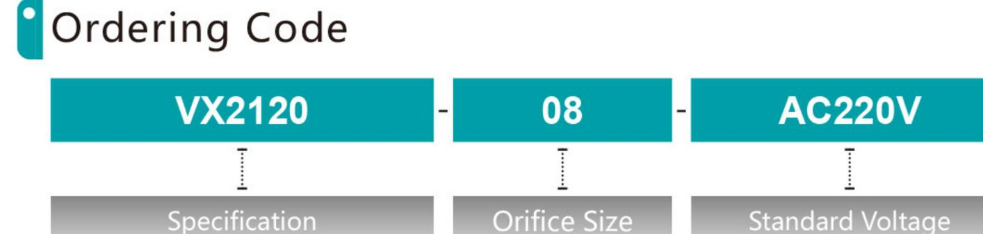
Wiring Orifice Size Standard Voltage 06: 1/8" DC24V J: Terminal DC12V W: Lead wire 08: 1/4" AC24V 50Hz/60Hz 10: 3/8" 50Hz/60Hz AC110V 15: 1/ 2" AC220V 50Hz/60Hz AC380V 50Hz/60Hz
